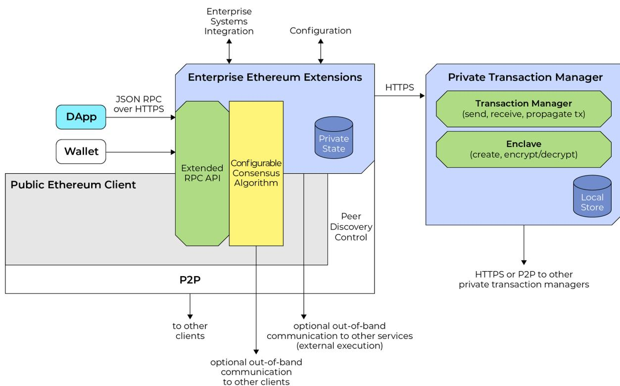
Figure 2. Representative Enterprise Ethereum High-level Architecture
