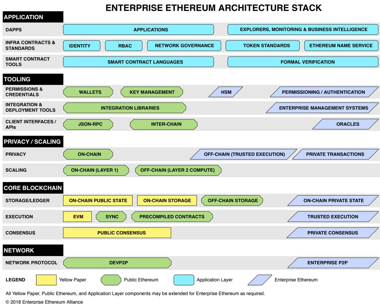
Figure 1. Enterprise Ethereum Architecture Stack
